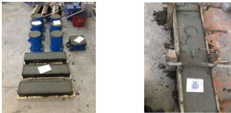
Figure (2): Casting of specimens
