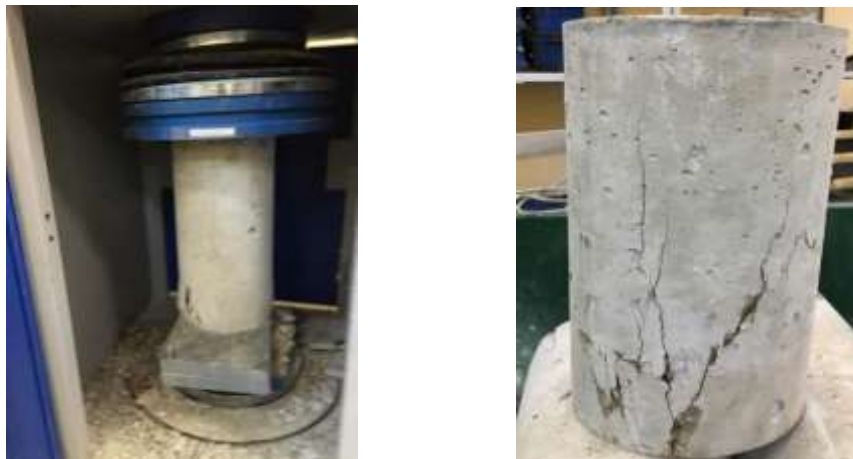
Figure (3): Compressive strength test for cylinder.
